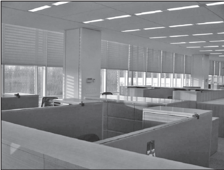
Exterior and interior views of the New York Times full-scale building mockup. The interior view shows the shades deployed to the lower edge of the upper exterior shading rods.
