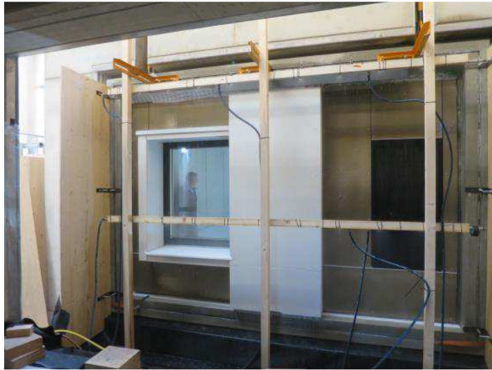
Fig. 10: Setup for the driving rain test (picture source: TU Graz)
