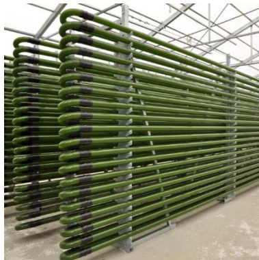
Tubular glass photobioreactor for the cultivation of microalgae Source: Wikimedia (IGV Biotech - licensed under CC BY-SA 3.0)
