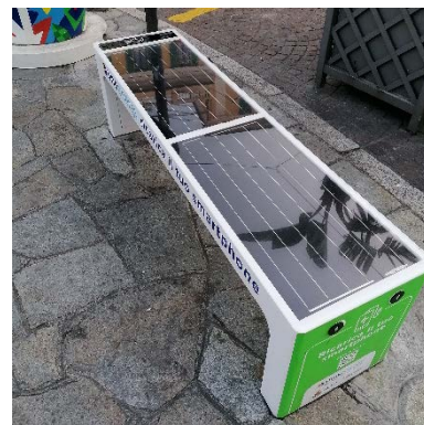
PV-integrated bench for the recharge of smartphones in a public squares - Sanremo (Italy) Photo: S. Croce
