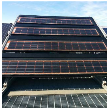
Experimental installation, photovoltaic-thermal solar panels for a solar-assisted heat pump. - Politecnico of Milan (Italy) Source: Wikimedia (Rich Schiz - licensed under CC-BY-SA 4.0)
